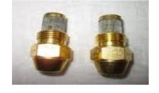
ACC & PCC line nozzles were of 36 GPH leading to higher fuel consumption. Fuel consumption was 540 KL.
